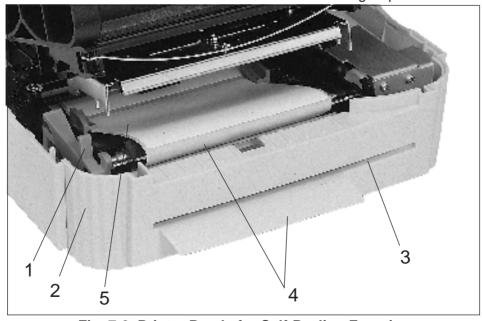
Fig. 7-2 Printer Ready for Self-Peeling Function
